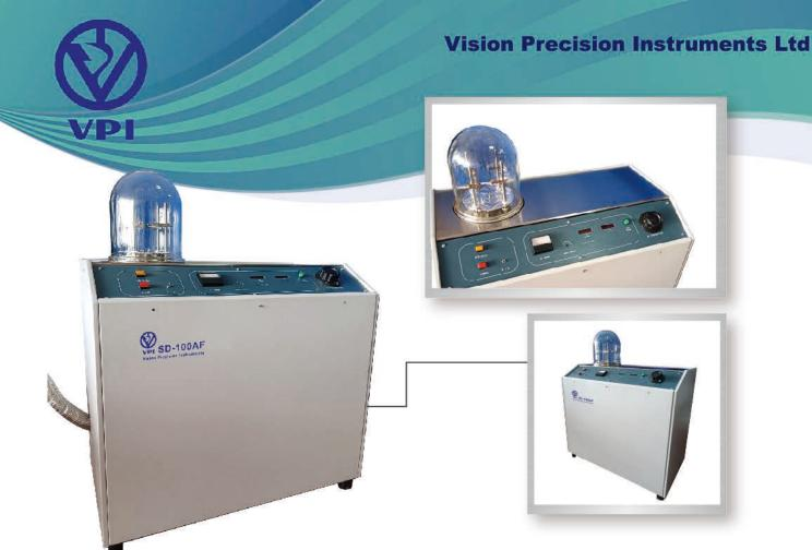
High Vacuum Thermal Evaporation Carbon Coater Model: SD-100AF
